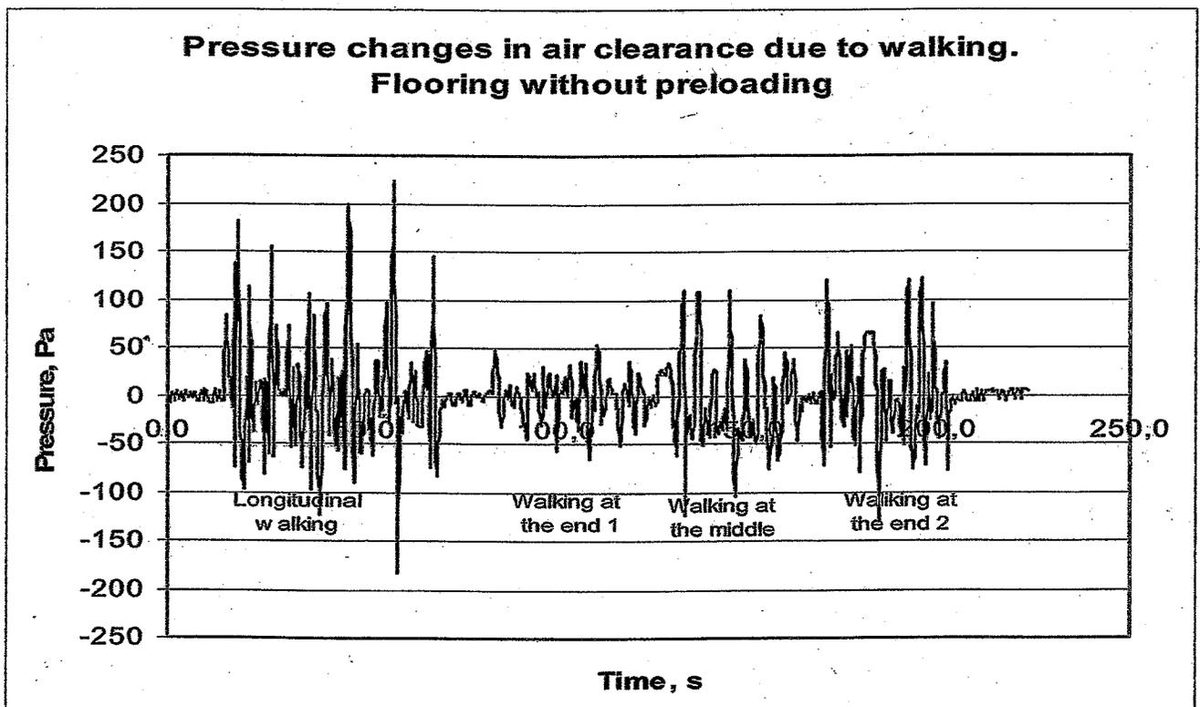
Figure 1. Pressure changes in air clearance due to walking. Flooring without preloading.
