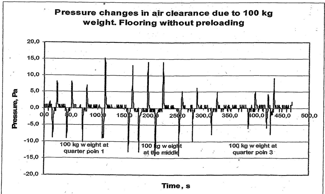
Figure 3. Pressure changes in air clearance due to 100 kg weights. Flooring without preloading.
