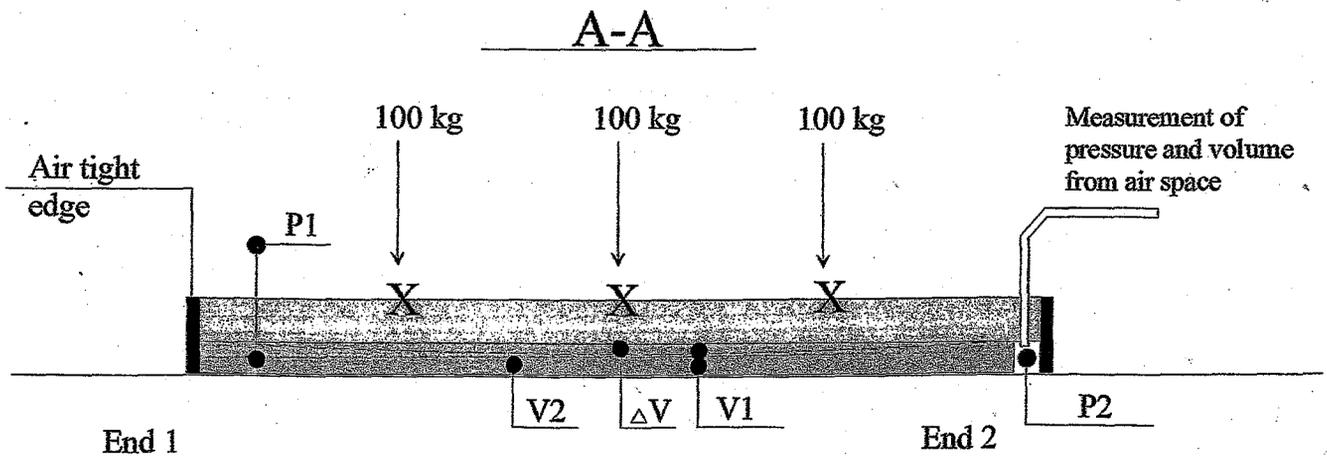
All the borders were tightened with sealing compound and laths
